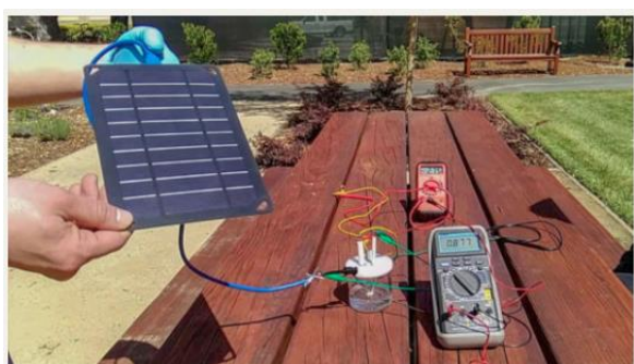
Hongjie Dai and his research lab at Stanford University have developed a prototype that can generate hydrogen fuel from seawater. (Image credit: Courtesy of H. Dai, Yun Kuang, Michael Kenney)
