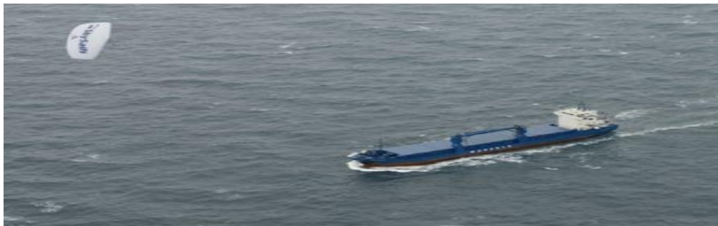
Fig 1. SkySails system installed on freight vessel “MV Michael A.”
