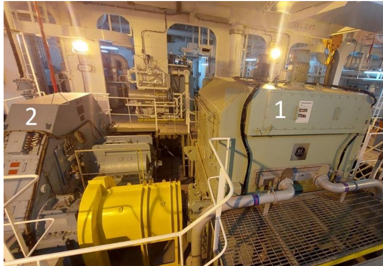
Figure 5. 1) propulsion motor, 2) Reduction gearbox (Source: Authors` personal collection)
